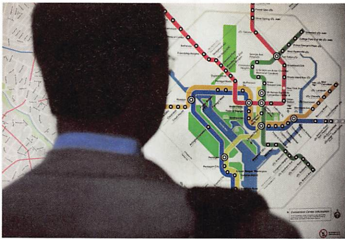
Figure 1.20 A traveler viewing a schematic network map of the Washington, DC, Metro system. The schematic network clearly shows train lines and connections at stations, essential for using the Metro system, but omits quantitative information about distances and directions along the system lines that are of little use to most riders.
