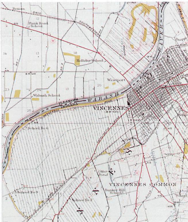
Figure 7.26 A portion of the Vincennes, Indiana-Illinois, topographic quadrangle (1944) showing evidence of the original French long-lot survey. Note the importance of the Wabash River in both long-lot and Vincennes street-system orientations. This U.S. Geological Survey map was originally published at the fractional scale of 1:62,500.
