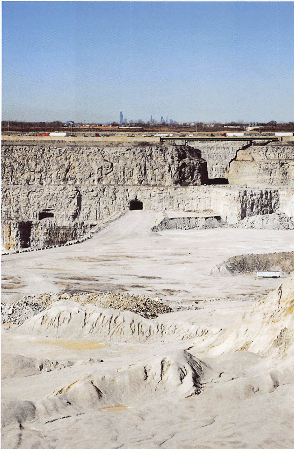
Figure 8.32 The Thornton quarry south of Chicago, depicted here with the city skyline in the distance, is one of the largest aggregate quarries in the world. It produces crushed limestone rock for road base and concrete mixes. Proximity to the market is necessary for low-value nonmetallic minerals unable to bear high transportation costs.
