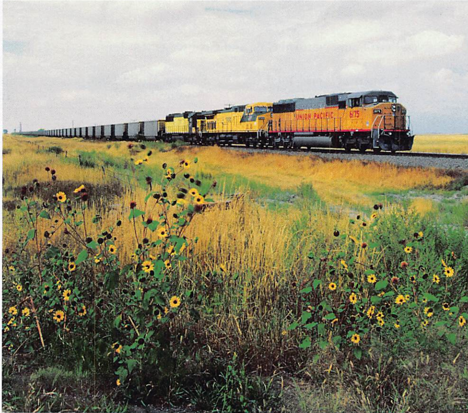
Figure 8.33 Long-distance transportation to eastern markets adds significantly to the cost of the low-sulfur western coal useful in meeting federal environmental protection standards. To minimize these costs, unit trains carrying only coal engage in a continuous shuttle movement between western strip mines and eastern utility companies.
