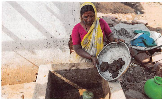
Figure 10.7 A woman adds waste to a biogas generator in Nepal. Human, animal, and vegetable wastes are significant energy sources in developing economies such as Pakistan, India, Thailand, and China, where such wastes are fermented to produce methane gas ( biogas ) as a fuel for cooking, lighting, and heating. The simple technology involves only a fermentation tank (foreground) fed with wastes—straw and other crop residues, manure, human waste, and kitchen scraps. These are left to decompose and ferment; the emitted methane gas passes into a large collection chamber and later is drawn through a tube into the farm kitchen. The remaining sludge is used for fertilizer in the fields.
