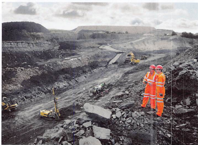
Figure 13.18 This open-pit coal mine in Scotland dramatically altered the landscape. On flat or rolling terrain, strip mining leaves a landscape of parallel ridges and trenches, the result of stripping away—overburden—the unwanted surface material. Besides altering the topography, open-pit mining interrupts surface and subsurface drainage patterns, destroys vegetation, and places sterile and frequently highly acidic subsoil and rock on top of the new ground surface.
