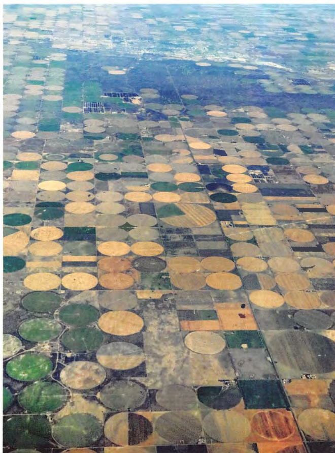
FIGURE 11.18 Great Plains, United States. The square pattern of land ownership found in the township and range land survey system marks farmland and towns as you fly over the Great Plains. The circles are from center-pivot irrigation systems.
